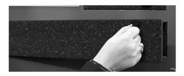
3. Pull out soiled filters. Remove filter support.
