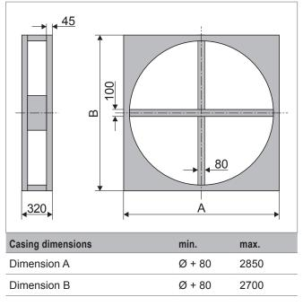
Table 6: Dimensional drawing for large sheet-metal casing, wheel diameter up to 1800 mm (dimensions in mm)
