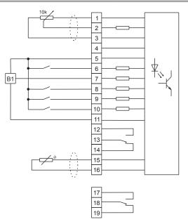
+10 V reference voltage Analogue setpoint input GND (analogue) Analogue output +15 V (max. 100 mA) Start clockwise External sensor Priority speed Parameter set switching Release GND (digital) Relay output 1 (normally open contact) Relay output 1 (changeover contact) Relay output 1 (normally closed contact) PTC motor temperature monitoring PTC motor temperature monitoring
