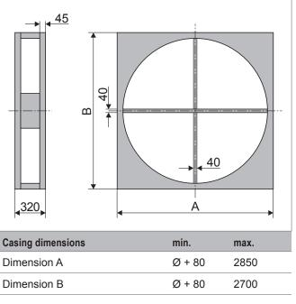
Table 8: Dimensional drawing for large sheet-metal casing, wheel diameter from 1800 mm (dimensions in mm)
