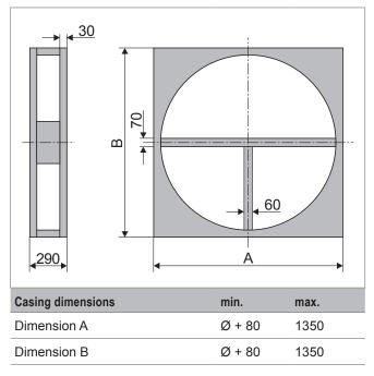
Table 5: Dimensional drawing for small sheet-metal casing (dimensions in mm)
