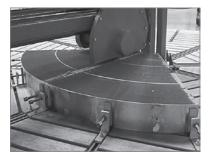
Fig. 9: A corrugated and a smooth metal foil are wound around each other.
