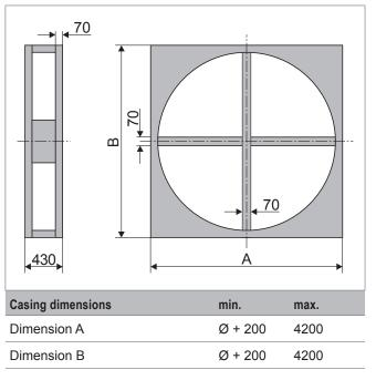
Table 7: Dimensional drawing for profile casing (dimensions in mm)
