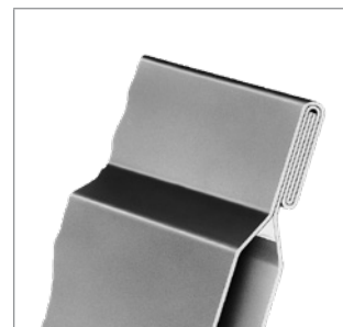
Fig. C3: Folded connections give the exchanger package several-fold material thickness for the leading and trailing edges
