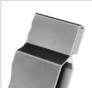
Fig. D3: Folded connections give the exchanger package several-fold material thickness for the leading and trailing edges
